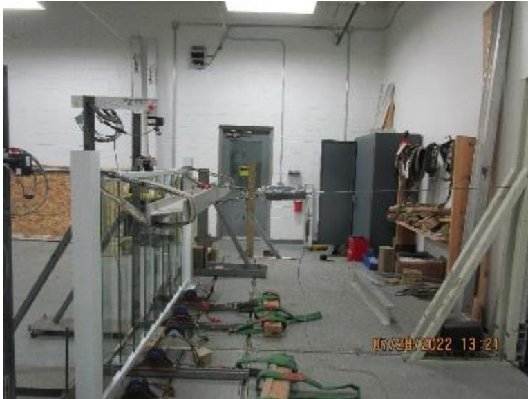
Photo No. 11 Horizontal Concentrated Load at Ends of Rail (Brackets)
