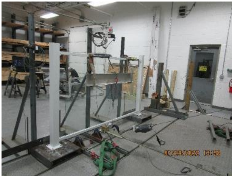
Photo No. 8 Vertical Uniform Load on Top Rail
