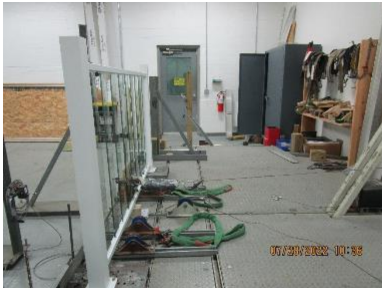
Photo No. 2 In-Fill Load Test at Bottom of Two Balustrades
