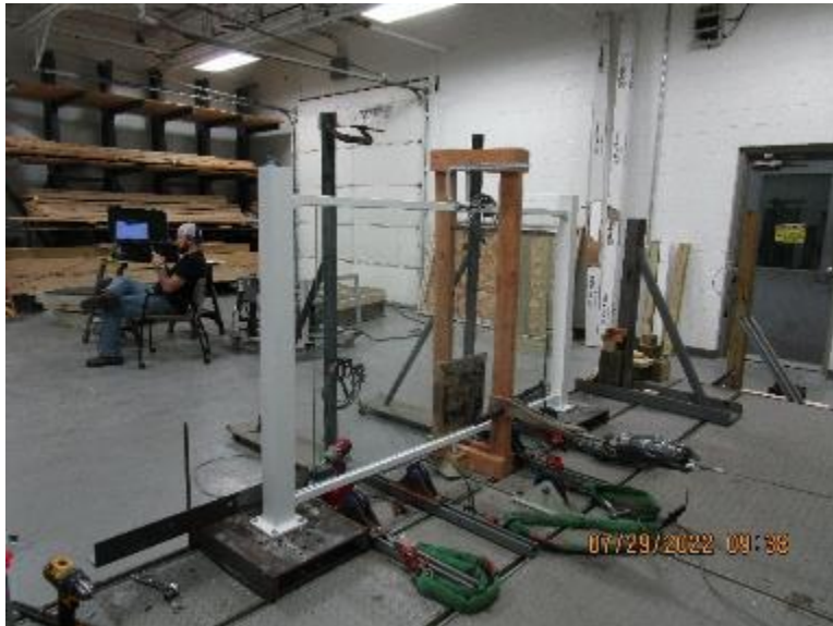
Photo No. 4 In-Fill Load Test at Bottom of Glass Panel
