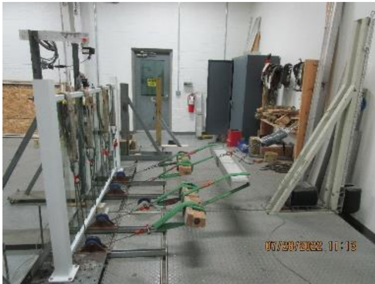
Photo No. 7 Vertical Uniform Load on Top Rail
